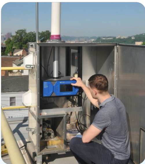
PM 2.5 monitor being checked to see that it is reporting live.
