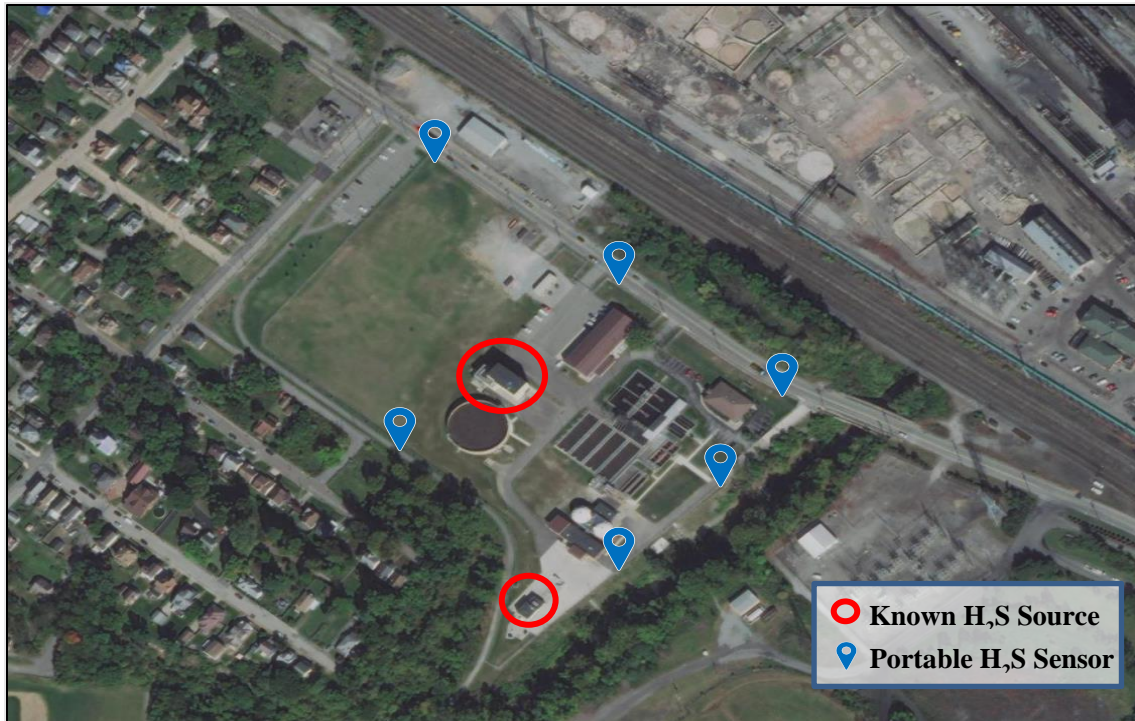
Figure 3.8: Location of known H 2 S sources at the Clairton Wastewater Treatment Plant and the portable H 2 S sensors installed by ACHD on the fence line of the property.
