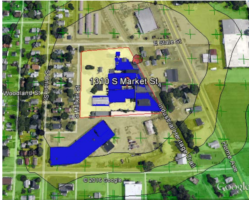
Figure 1. Simulation using 500 degrees K exit temperature. Blue indicates building included in downwash simulation. Peak receptor area is identified in red. Light green to darker green indicates decreasing concentrations.
