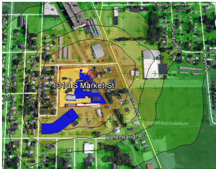
Figure 2. Simulation using 1000 degree K exit temperature. Blue indicates building included in downwash simulation. Peak receptor area is identified in red. Light green to darker green indicates decreasing concentrations.
