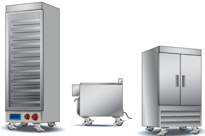
Figure 1 - Kitchen Equipment Mounted on Casters
