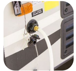
Filling a water supply tank with a food grade hose.
