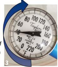
temperature and make any adjustments. Twist the thermometer head so that it shows 32° F.
