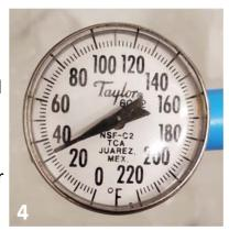
reads the right temperature in ice water, it will give the correct reading at other temperatures, too.
